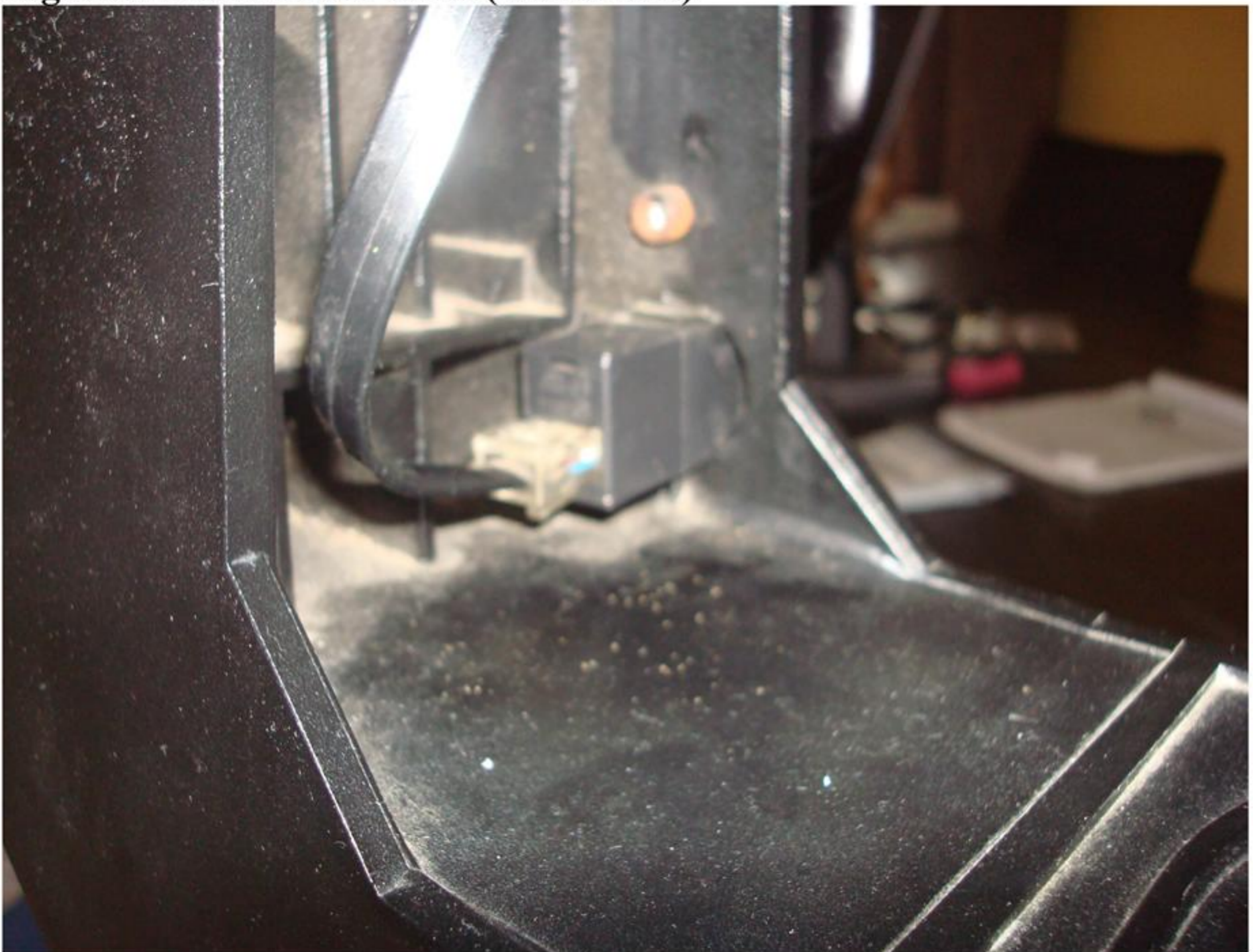
Unplug declination motor cable (inside fork)
